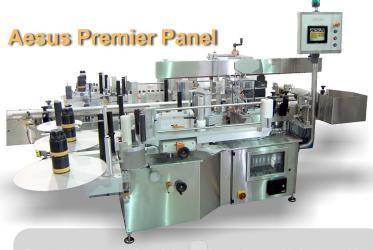
Front, back, 3panel and 4 panel and 5 panel labeling with speeds up to 200 per minute the Premier-Panel include the powerful Servo Herma 400 head(s) and a stainless base Cabinet, with stainless clad top plate.
