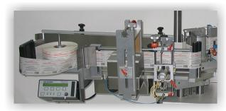
The heavy duty mounting plate is arranged conveniently along the length of the labeler so that it does not stick out into the aisle way. It is solid to give extra rigidity for preferred mounting of Coders and vision systems.
